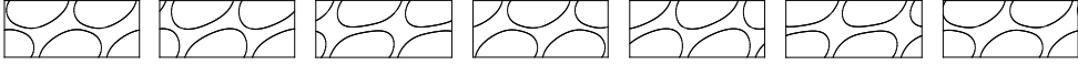
FIGURE 3. The temporal evolution of the bubble configuration for Ca=0.1 , Bi=0.1 and Pe = 1 (case B in table 1). The lines correspond to the liquid–gas interface, i.e. \phi = 0 . The first snapshot corresponds to \tilde{t}=1.82 and the time interval between two successive snapshots is \Delta\tilde{t}=0.19 .
